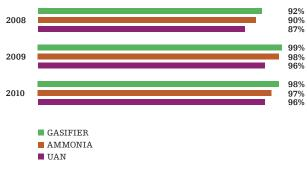
On-stream factor is the total number of hours operated divided by the total number of hours in the reporting period, excluding the impacts of major planned turnarounds in 2008 and 2010 and adjusted for a Linde air separation outage in April 2009 and a vessel rupture in the UAN plant in October 2010.
